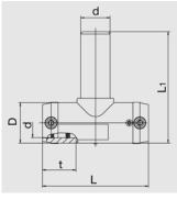
Straight connector with exposed heating coils for optimal heat transfer, large insertion depth, wide fusion zones plus cold zones at the end and in the middle to prevent the flow of molten material, for use without holding devices. Extra long outlet spigot dimensioned for 2 fusion operations (if necessary).
