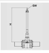
To operate the FRIALOC PE shut-off valve from the surface box. Optimally matched, can be individually extended to the required covering height. With KlickFix coupler for easy installation. Made of galvanised steel or stainless steel.
