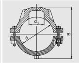
Compact part manufactured from 2 HD-PE saddles for the repair of minor pipe damage **with or without** escape of fluid. In order to avoid discharge of media the leak has to be sealed with a separate plug\* ( $\leq$  d3). With exposed heating elements for optimal heat transfer.
