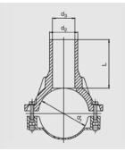
Compact part in HD-PE, saddle with exposed heating element for optimal heat transfer and outlet spigot for use with FRIALEN-couplers MB or UB. Swarfless tapping in the depressurised state by means of commercial drilling units (we recommend Hütz & Baumgarten (www.huetz-baumgarten.de)).
