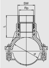
Compact part. In HD-PE, saddle with exposed heating element for optimal heat transfer. Gunmetal adapter permanently anchored in the HD-PE. To accept normal commercial brass valves.
