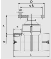
Compact part in HD-PE. Factory made combination made from FRIALEN-T-Piece, Reducer and Full Faced Flanges (fixed flange). T-Piece with exposed heating coils for optimal heat transfer, large insertion depth, wide fusion zones plus cold zones at the end and in the middle to prevent the flow of molten material for use without holding devices.
