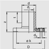
Flange Adaptor and flange as a factory made flange piece. Metal insert in the flange to prevent creep. Spigot end for use with FRIALEN-couplers MB or UB. Flange connection dimensions to DIN 2501, part 1. GST sealing recommended.
