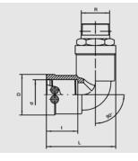
Compact part. HD-PE end with exposed heating coils for optimal heat transfer, large insertion depth, wide fusion zone plus cold zones at the end and in the transition area to prevent the flow of molten material for use without holding devices. Steel end permanently anchored in the HD-PE. Self sealing patented sealing geometry without elastomer seal. For use in gas systems.
