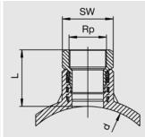
Suitable for all pipe diameters in the given range by means of the FRIALEN-FRIATOP Clamping Unit (see Product Range FRIATOOLS Technical Equipment). HD-PE saddle with exposed heating element for optimal heat transfer. Gunmetal adapter permanently anchored in the HD-PE. To accept normal commercial brass valves.
