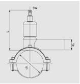
Compact part in HD-PE with no threaded connections. Actuating spindle in stainless steel 1.4305. No re-insulating required. Leak free and swarfless tapping up to 10 bar (gas) or 16 bar (water). Integral drill with upper and lower stop, guided in a metal sleeve. With exposed heating element for optimal heat transfer. Maintenance free, operating isolating valve actuated by a linkage (e.g. FRIALEN EBS). Length of the outlet spigots dimensioned for 2 fusion operations (if necessary).
