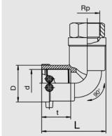
Compact part. HD-PE end with exposed heating coils for optimal heat transfer, large insertion depth, wide fusion zone plus cold zones at the end and in the transition area to prevent the flow of molten material for use without holding devices. Steel end permanently anchored in the HD-PE. Self sealing patented sealing geometry without elastomer seal. For use in gas systems.
