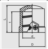
With exposed heating coils for optimal heat transfer, large insertion depth, wide fusion zone plus cold zones at the end to prevent the flow of molten material.
