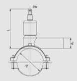
Compact part in HD-PE with no threaded connections. Actuating spindle in stainless steel 1.4305. No re-insulating required. Leak free and swarfless tapping up to 10 bar (gas) or 16 bar (water). Integral drill with upper and lower stop, guided in a metal sleeve. With exposed heating element for optimal heat transfer. Maintenance free, operating isolating valve actuated by a linkage (e.g. FRIALEN- EBS). Length of the outlet spigot dimensioned for 2 fusion operations (if necessary).
