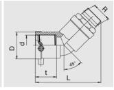
Compact part. HD-PE end with exposed heating coils for optimal heat transfer, large insertion depth, wide fusion zone plus cold zones at the end and in the transition area to prevent the flow of molten material for use without holding devices. Brass end permanently anchored in the HD-PE. Self sealing patented sealing geometry without elastomer seal. For use in water systems.
