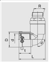
Compact part. HD-PE end with exposed heating coils for optimal heat transfer, large insertion depth, wide fusion zone plus cold zones at the end and in the transition area to prevent the flow of molten material for use without holding devices. Brass end permanently anchored in the HD-PE. Self sealing patented sealing geometry without elastomer seal. For use in water systems.
