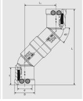
Compact part for the connection of pipes which are not aligned and for the connection of service lines with DAA pressure valves when parallel-installing two mains with identical overlap height. With exposed heating coils for optimal heat transfer, large insertion depth, wide fusion zone plus cold zones at the end and in the transition area to prevent the flow of molten material for use without holding devices.
