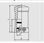
With exposed heating coils for optimal heat transfer, large insertion depth, wide fusion zone plus cold zones at the end to prevent the flow of molten material, for use without holding devices. From d 180 with fusion indicators for visual fusion control.
