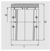
With exposed heating coils for optimal heat transfer, large insertion depth, wide fusion zones plus cold zones at the end and in the middle to prevent the flow of molten material, for use without holding devices. From d 250 with fusion indicators for visual fusion control.
