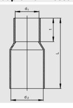
For fitting on the square drive of the FRIALEN-DAV for adaptation to the standard commercial linkage with 50 mm guard tube.
