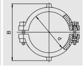
Compact part manufactured from 2 HD-PE saddles for the repair of minor pipe damage **with no** escape of fluid. With exposed heating elements for optimal heat transfer.
