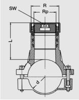
Compact part suitable for normal commercial shut off equipment. HD-PE saddle with exposed heating element for optimal heat transfer. Brass-guide thread permanently and immovably anchored in the HD-PE. Includes brass plugs with square recess. Protection against access to the dome by fusing on a FRIALEN-SPAK (when using d 63 through cap K). Thread to DIN ISO 228.
