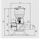
For connection of hydrant with cast spigot. Compact construction part manufactured from FRIALEN 90° elbow with base (see WF 90°) and NOVO-Sit coupler connection made from ductile cast iron including Tyton sealing ring and NOVO-Sit ring for push prevention. NOVO-Sit cast coupler anchored in PE moulded part. Cannot be released or rotated. Please observe specific processing instructions for "NOVO-Sit" connection system.
