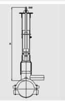
Telescopic actuating linkage for operation of the FRIALEN-DAV from the street cap. Stepless adjustment in the stated range (H) without the use of tools, even in the installed state. Self supporting in any extended position. Corrosion proof.
