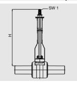
Telescopic actuating linkage for operation of the FRIALEN-KHP, KH, AKHP and AKHP-TL from the valve cover. Stepless adjustment in the stated range (H) without the use of tools, even in the installed state. Self supporting in any extended position. Corrosion proof. **Key width 14 version specially designed for domestic connection.**
