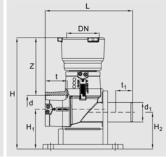
For connection of hydrant with spigot according to BAIO system as alternative to flange connection. Compact construction part manufactured from FRIALEN 90° elbow with base (see WF 90°) and BAIO coupler connection made from ductile cast iron including sealing ring. BAIO cast coupler anchored in PE moulded part. Cannot be released or rotated. Please observe specific processing instructions for "BAIO" connection system.
