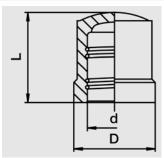
With exposed heating coils for optimal heat transfer, large insertion depth, extra wide fusion zone plus cold zones at the end to prevent the flow of molten material.
