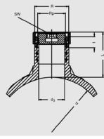
Suitable for all pipe diameters in the given range by means of the FRIALEN-FRIATOP Clamping Unit (see Product Range FRIATOOLS Technical Equipment). Compact part to accept normal commercial bubble setting units. HD-PE saddle with exposed heating element for optimal heat transfer. Brass guide thread permanently anchored in the HD-PE. Includes brass plugs with a square recess. Access protection for dome through screw-cap flap supplied or through welding on of a FRIALEN-SPAK. Thread to DIN
