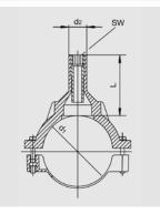
Compact part in HD-PE, saddle with exposed heating element for optimal heat transfer and outlet spigot for use with FRIALEN-couplers MB or UB. Swarfless tapping in the depressurised state by means of the integral drill.
