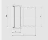
Flexible material transition in domestic range between HD-PE pipes (SDR 33 - SDR 17) and PVC/PP pipes. HD-PE side can be fused with FRIAFIT AM sewage coupler or with the outlet of the FRIAFIT ASA-TL sewage saddle. PVC/PP side acts as push-fit coupler with SBR lip seal gasket and large insertion depth.
